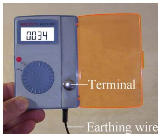
One of the terminals of the meter is touched with a finger, while the other terminal connects to a wire (Earthing wire) that connects to a rod in the Earth or to a good ground in the electrical system. It is important that the body voltage meter has the capability to measure the AC electrical potential between your skin and the surface of the Earth.
